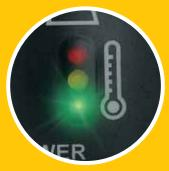
Temperature gauge alerts operator if motor overheats to help prevent unnecessary burnout. NOTE: Operation manual shows operators step by step how to run the cool-down cycle
