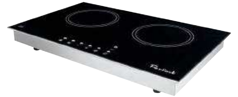
Induction Plate Double IP 8200 Size: 665 x 405 x 85mm Power 1.65kw +1.65kw Voltage 220V 1NAC Current 7.5 A Timer 1~99 minutes
